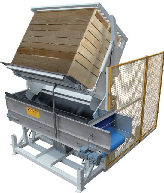
Box tipper with discharge conveyor in the tipping position
